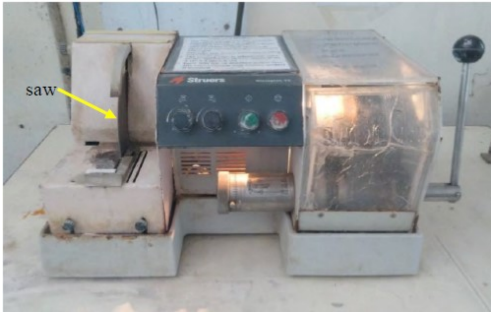
Diamond tipped saw used in the study to cut thin slices of samples
