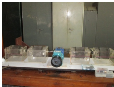
Apparatus for dynamic testing of acid attack
