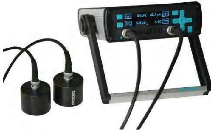
Pundit lab instrument for measuring ultrasonic pulse velocity – can be used in studying the property change after acid attack
